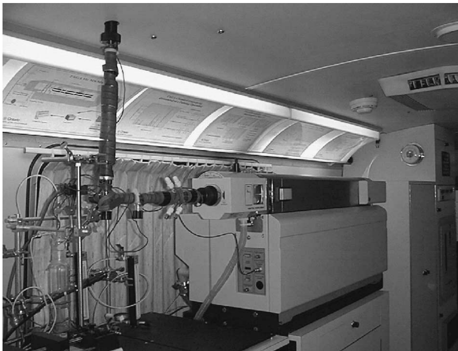
Fig. 2. The TAGA IIe mass spectrometer housed inside the mobile analytical laboratory, known as the “Explorer”.
